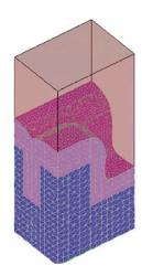
Geometry defined using sheet surfaces as material interfaces. The top material is transparent so that the finely-gridded moving surface is visible. The history of a previous time step is visible in the surface trace in the "pink" material.
