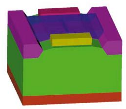
Semiconductor device modelcomputational grid is generated from solid model. Note clean interfaces between materials, varied aspect ratios of elements, and use of proportional spacing in the green silicon region.
