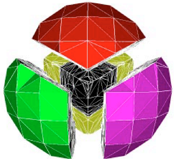
Fig. 2: Configuration at t = 0.1 after evolution by surface tension (using Moving Finite Elements for Surfaces). Interfaces are smoothed; central grain has become a curved tetrahedron.
